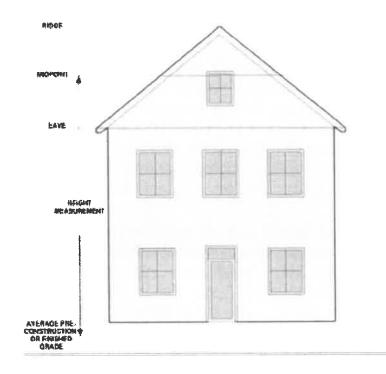
Gable or Hip Roof. Height is measured to the midpoint between the caves and the ridge, regardless of the orientation of the gable to the street.
