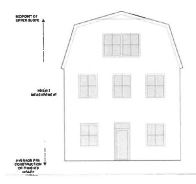
Gambrel Roof. Height is measured to the midpoint of the uppermost slope of the
